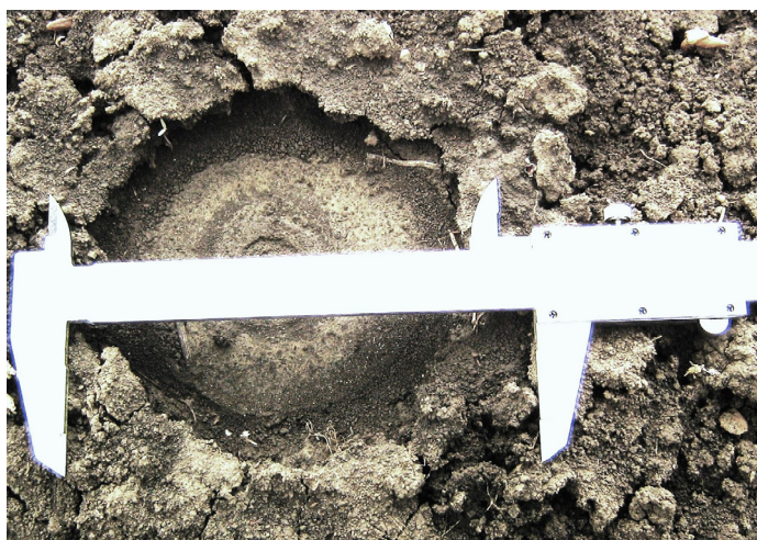
Figure 2. Typical circuit moisture under drip irrigation of an orchard
