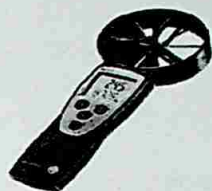
3.6.4-rasm. Havo harakat tezligini o'lchovchi parrakli anemometr
